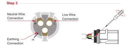
Connect AC Line, Live Line (L), Neutral Line (N) and Ground Wire (PE) according to polarity.
