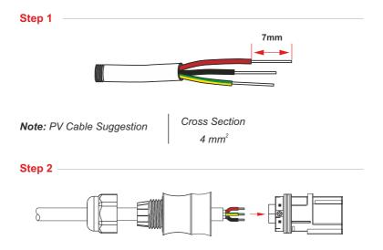
Note: AC line goes through AC terminal waterproof head and cap
