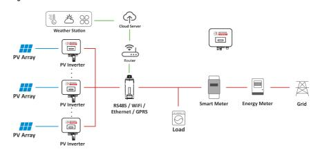
Note: The Inverter could be connected in parallel with Smart Meter, make sure the total load power does not exceed Smart Meter's limitation.
